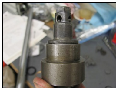
Ring Compressor (upside down) Covering Piston Rings on Damper Rod
