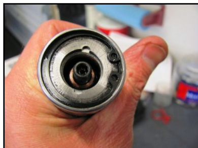
Snap Ring at Bottom of Fork Tube with Damper Rod in Center
