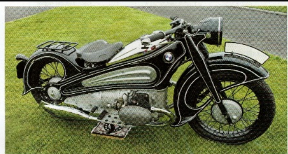
Once thought lost, this 1934 BMW R7 concept bike was found after some 70 years in storage and restored by BMW, which still owns the splendid machine and showed it at Pebble Beach as part of its 100th anniversary celebrations. Not just streamlined and stunning, the R7 also featured a monocoque steel structure, an innovative engine and BMW's first use of telescopic forks.
