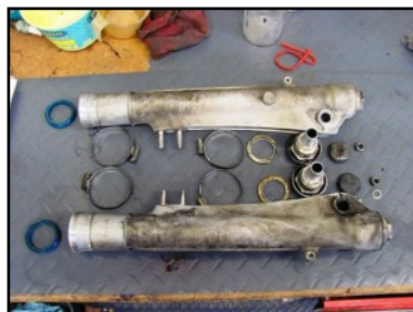
Left - Fork slider Parts and Fork Tube Top Retaining Caps
