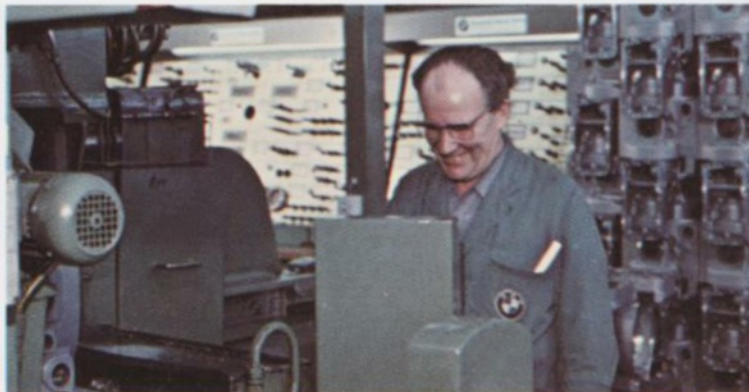
Crankshaft runout readings are displayed and recorded. Vast control board at rear signals any tolerance error.
