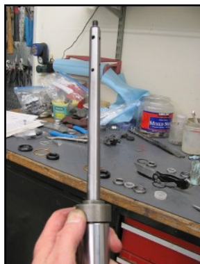
Damper Rod with Compressor Inserted into Fork Tube
