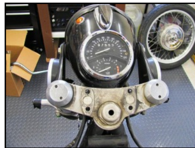
Handlebars Removed Showing Chrome Covers Over Fork Spring Nuts
