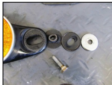
Headlight Ear Headlight Mount Detail
