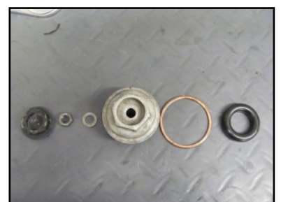
Bottom of Fork Slider, rubber cover, wave washer, 10 mm nut, fork plug, large copper ring, inner rubber bumper
