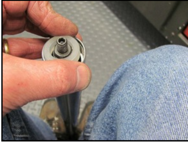
Inserting White Bumper into the Bottom of the Fork Tube
