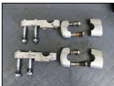
Handlebar Pullbacks and Original Handlebar Mounts
