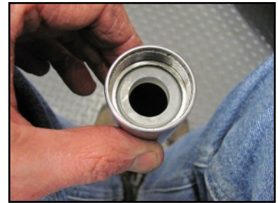
Bumper Stop Just Past Internal Threads
