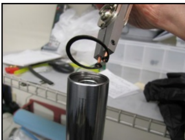
Inserting bottom snap ring
