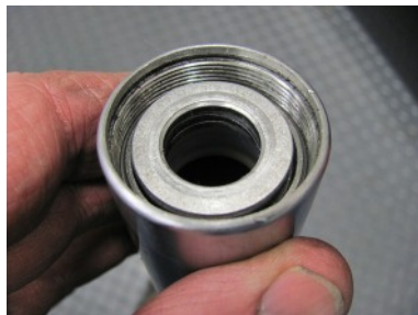
Metal Spacer Ring Inserted
