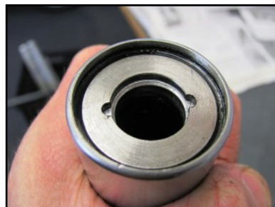
One Style of Retaining Ring-You Can't use Tool Kit Pin Wrench
